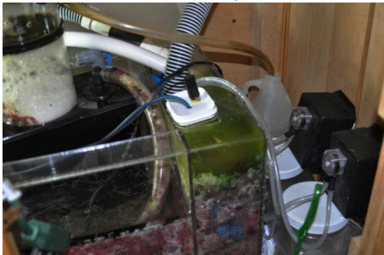
Drew's dosing pumps controlled by the Apex.
